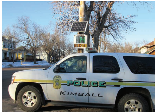
The speed meter is along Main Street. It shows the speed in red with "slow down" when a driver is speeding. It will be green and show "Thank You" for appropriate speeds as pictured.
