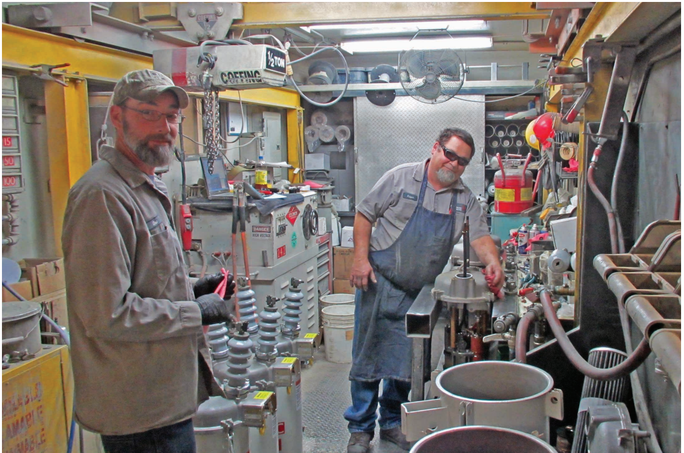
Employees from Solomon Corporation shown in their mobile workshop busy working to refurbish oil circuit reclosures for Central Electric.
