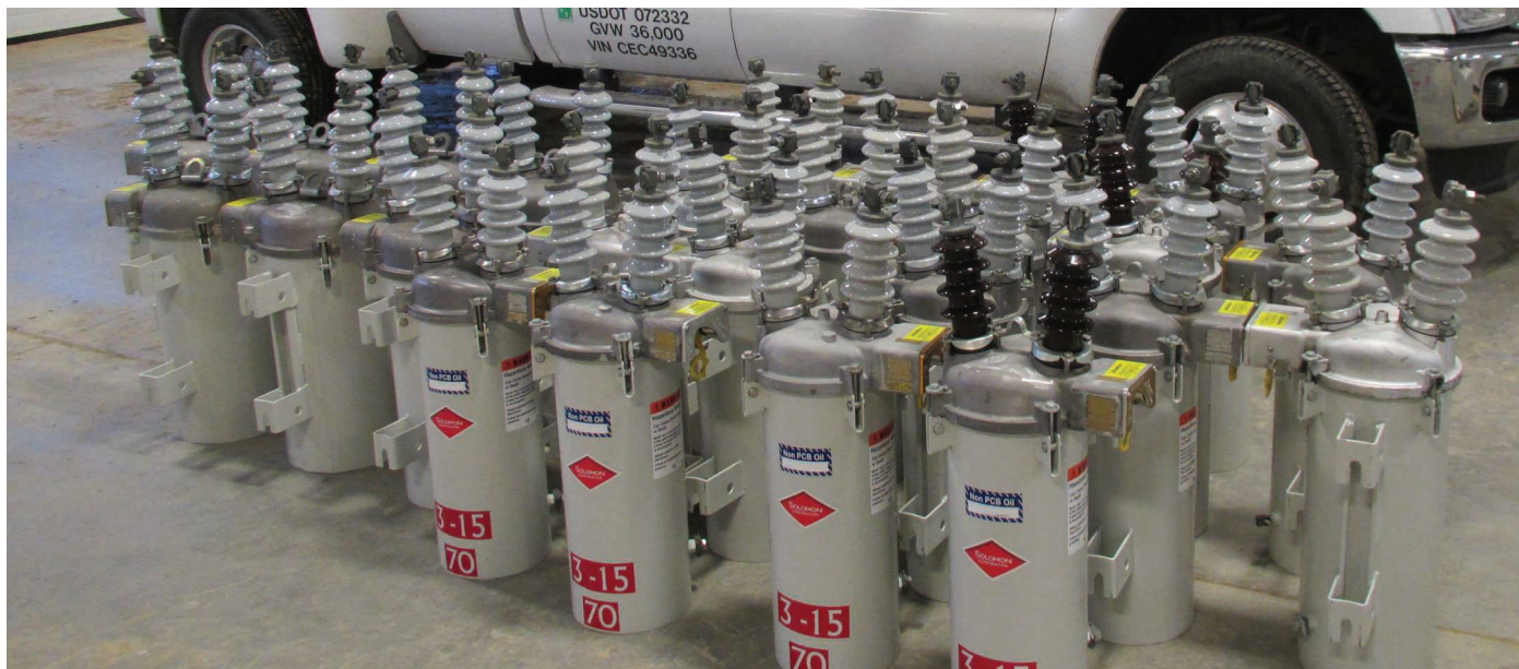
Rows of oil circuit reclosures that have been refurbished and ready to be placed back in service by Central Electric crews.
