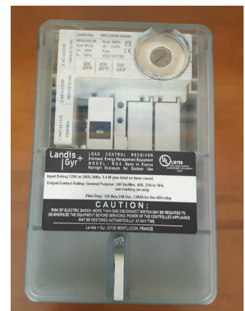
Below: This is a new load management receiver that will be installed. Some members may already have these in their homes.
